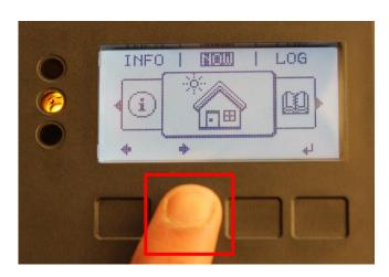
Enter the inverter's **Setup** function by pressing the fourth button.
